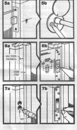
It is important to use all parts supplied with this lock on your installation to comply with BS 3621:2007. If the lock requires lubricating use only a proprietory maintenance fluid (e.g WD40) not oil.
